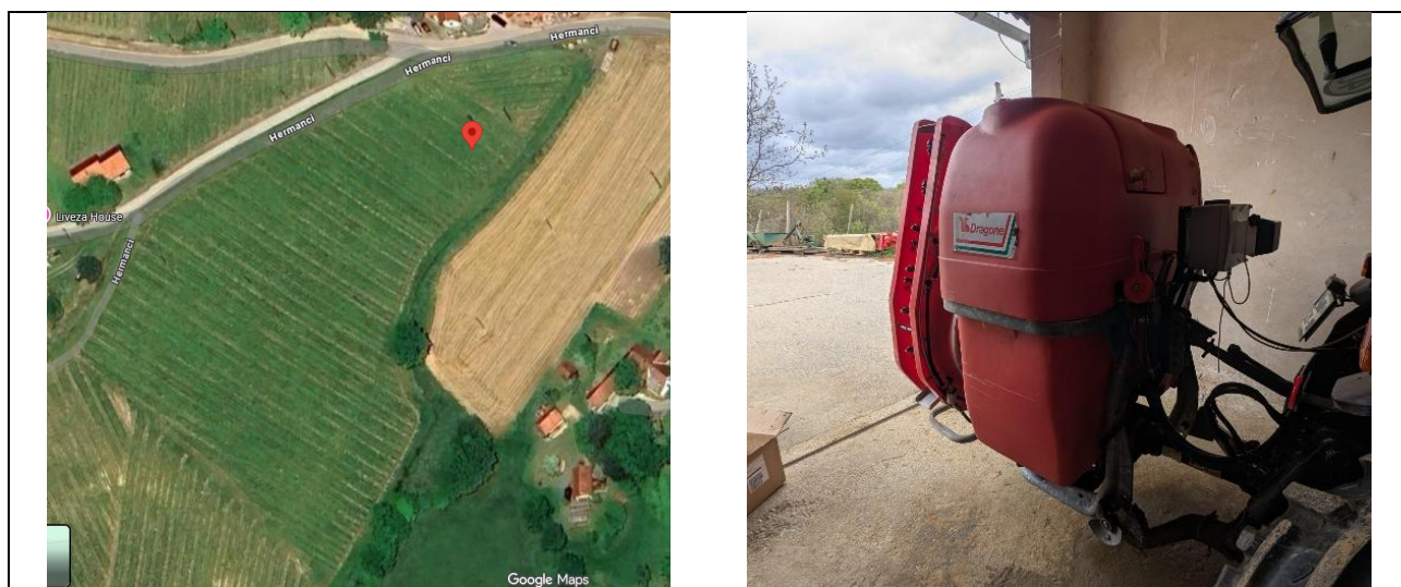
Fig. 1. Overview of the experimental site (left) and the modified conventional sprayer equipped with a real-time spray mixture control system (right).
