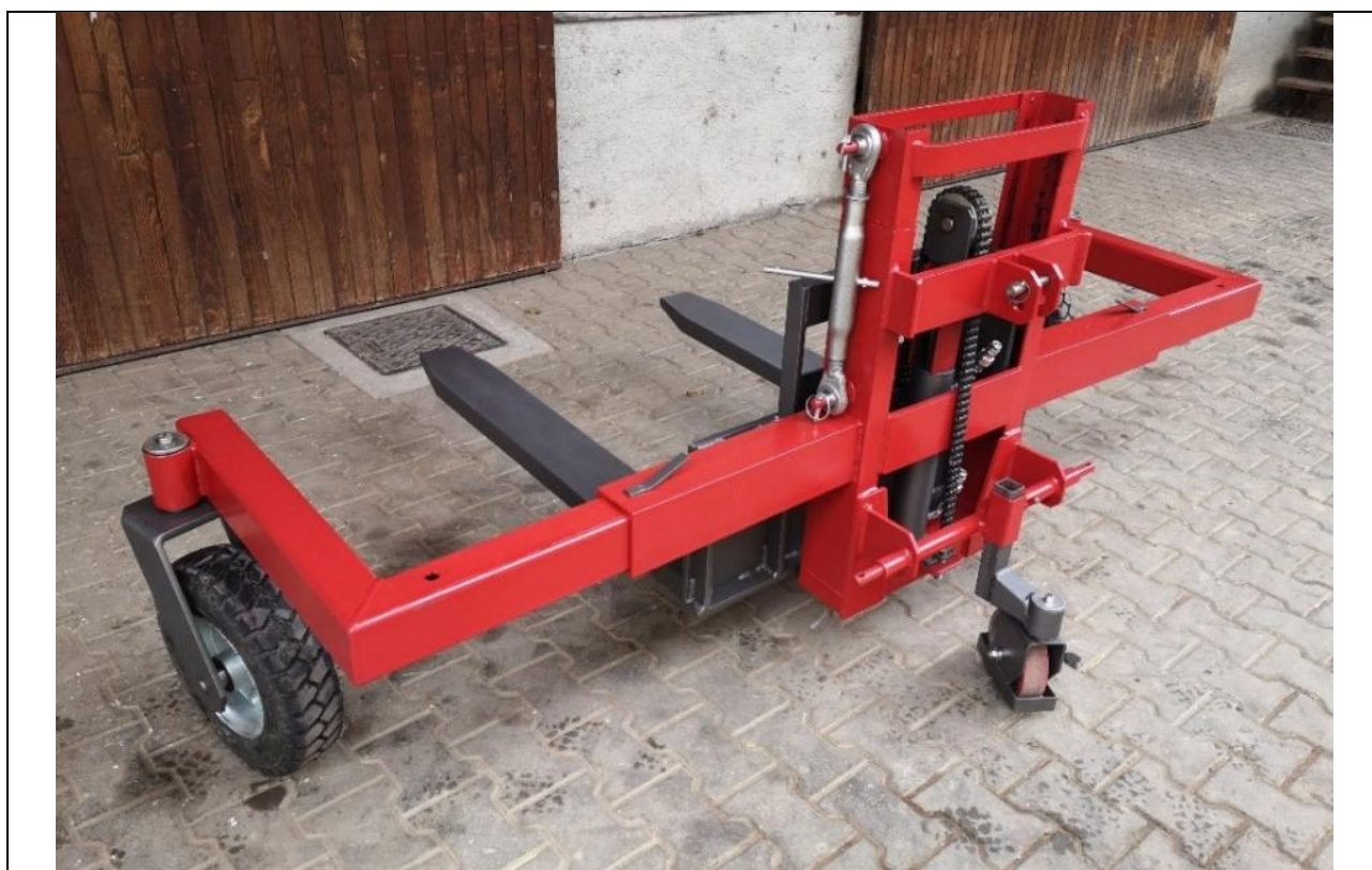
Fig. 5. Tractor forklift with extended telescopic arms.
