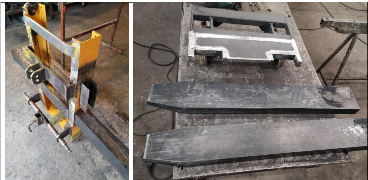
Fig. 4. Category one of three-point hitch (left) and fork modification (right).
