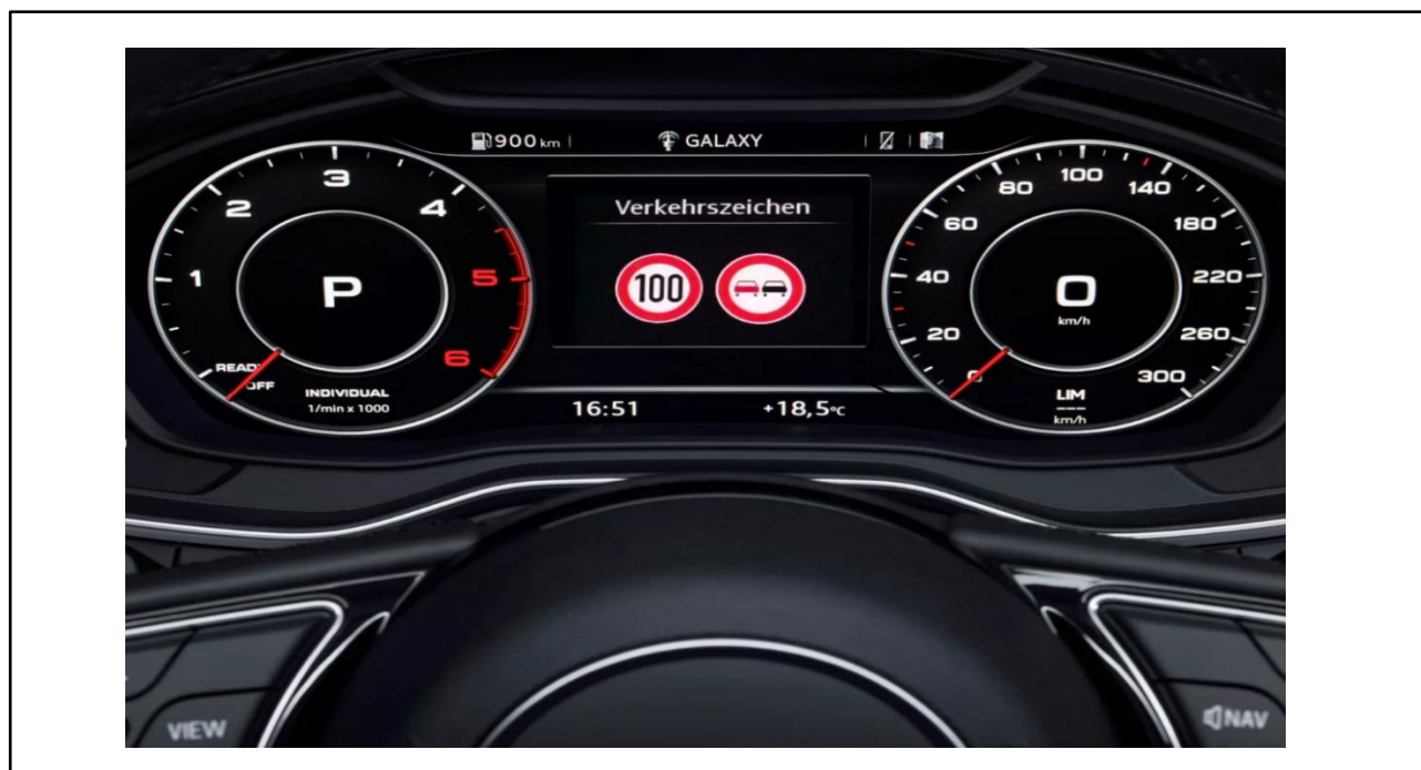
Fig. 10. Display of detected traffic signs using TSR
