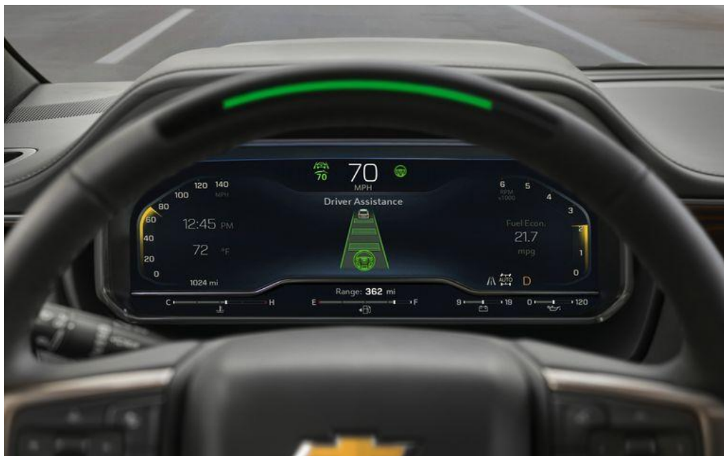
Fig. 13. GM Super Cruise technology lane keeping assist
