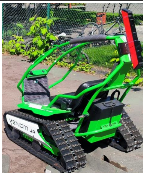
Fig. 2. Mobile logistics platform for testing sensor equipment and for training operators in remote control.
