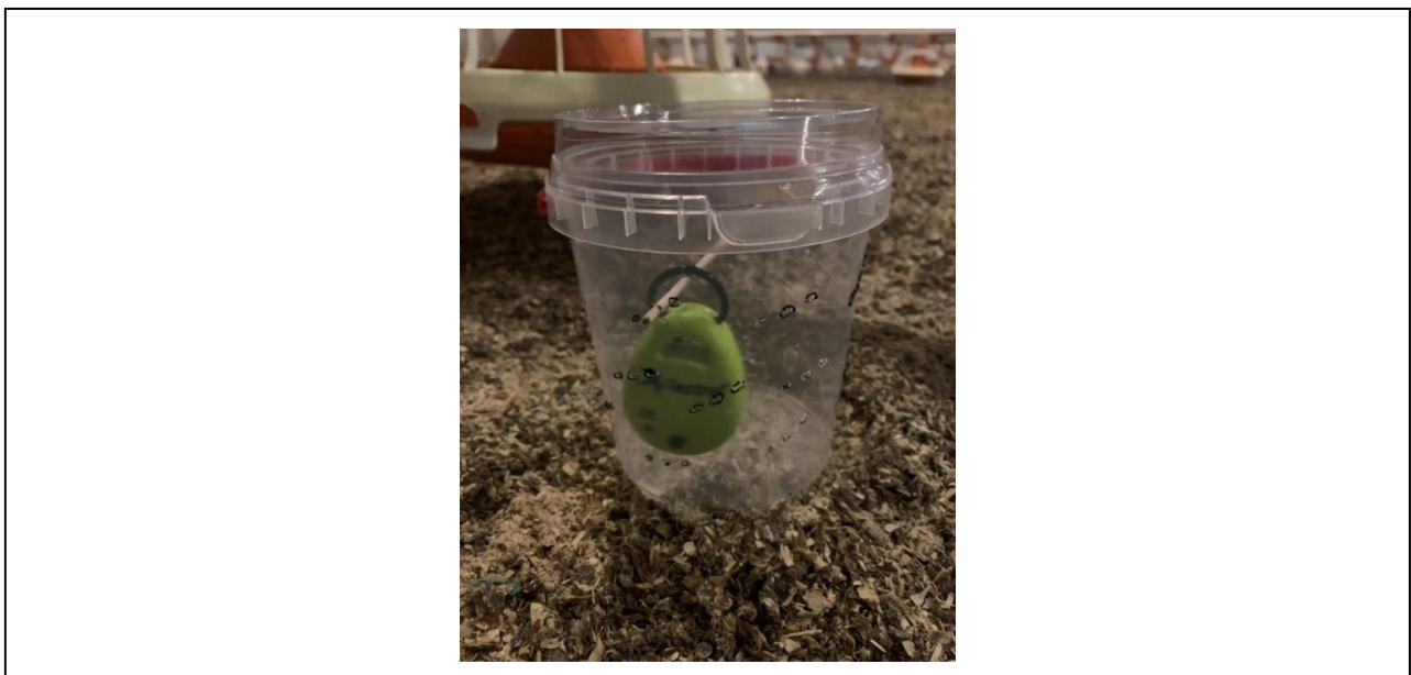
Fig. 5. The Kestrel DROP D2AG humidity and temperature air sensor (Levanic, 2021).
