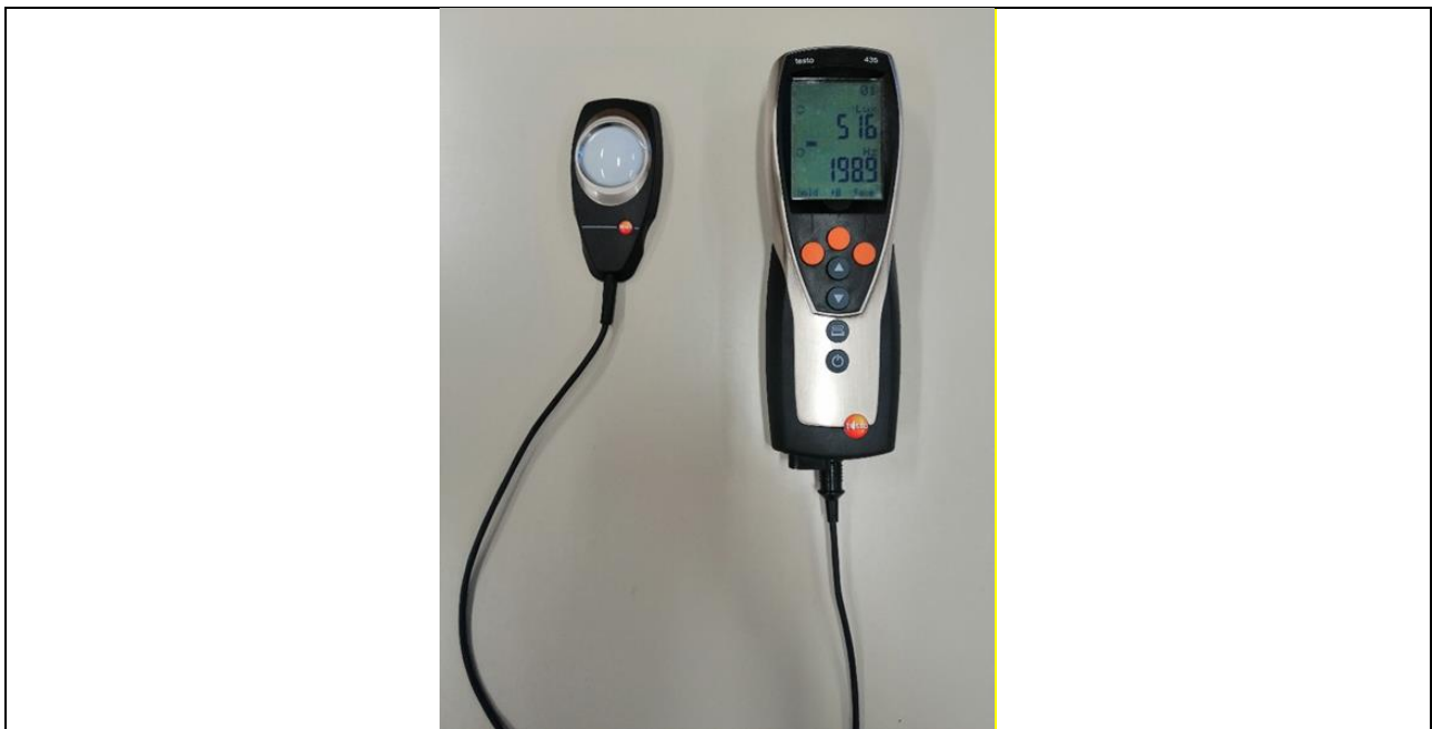
Fig. 2. Multifunctional measuring device Testo 435 (Testo SE & Co, Germany).
