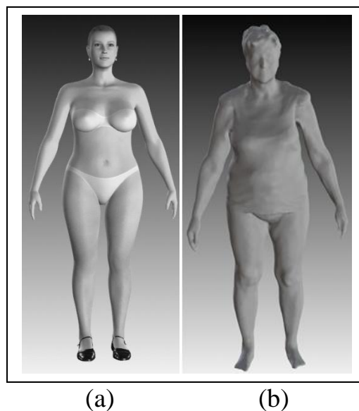
Fig. 1. Female virtual body model (a) parametric 3D body model, (b) scanned and reconstructed 3D body model
