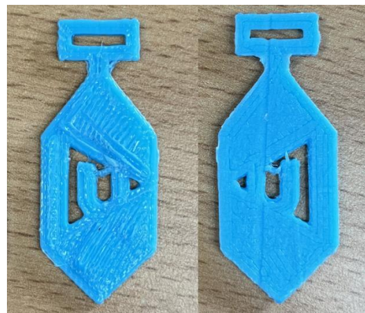
Fig. 10. Selected Dobot Magician keychain result using the PLA supplied with the robot.
