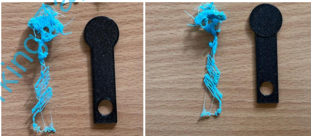
Fig. 4. Preliminary 0.2mm Speed trial: failed Dobot deposition (blue) and the Prusa specimen (black).
