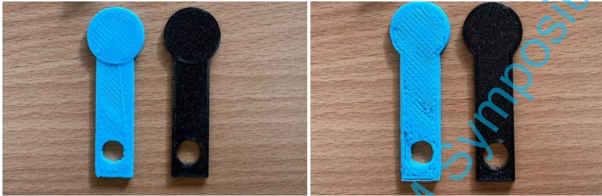
Fig. 5. Simple geometric specimens obtained with the recorded Dobot Best Setting: Dobot in blue and Prusa in black. Front view on the left and rear view on the right. The photographs were not calibrated for dimensional measurement.
