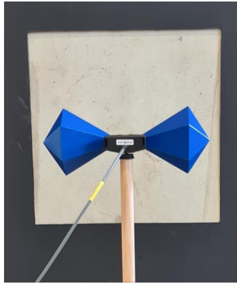
Fig. 2. Bicol antenna (operating frequency range: 50 MHz–1 GHz)
