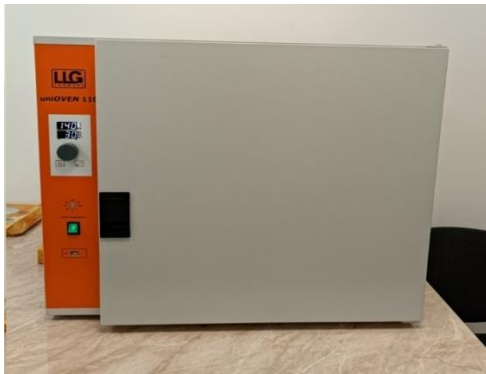
Fig. 5. Laboratory oven uniOVEN 110 used for thermal annealing and test specimens inside
