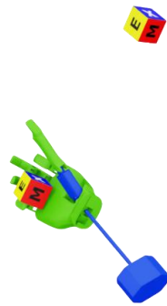
Fig. 10. 8-DoF Bionic Hand with wrist flexion/extension using the fast axes to orient the cube and keeping it in place with finger joints
