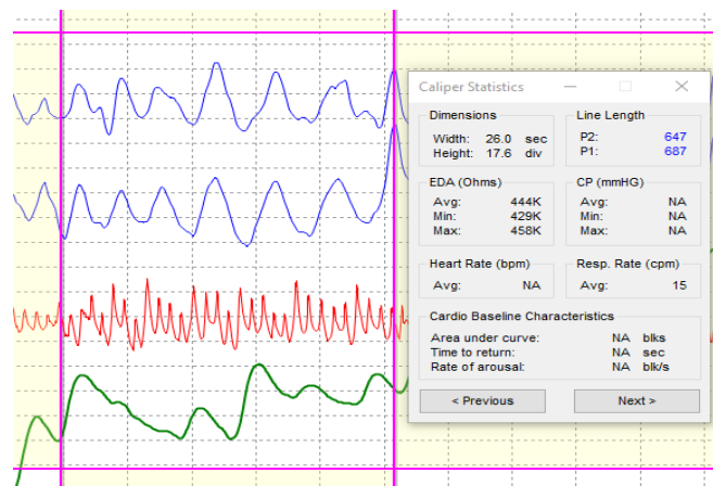
Fig. 3. The Caliper Statistics window displays the dimensions of the chart area selected by the calipers. This feature enables the measurement of distinct patterns in the obtained data.
