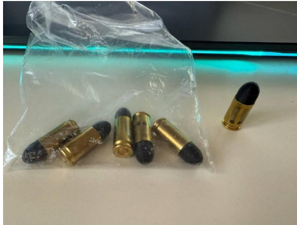
Fig. 3. 9 x 19 mm ammunition with polymer projectiles
