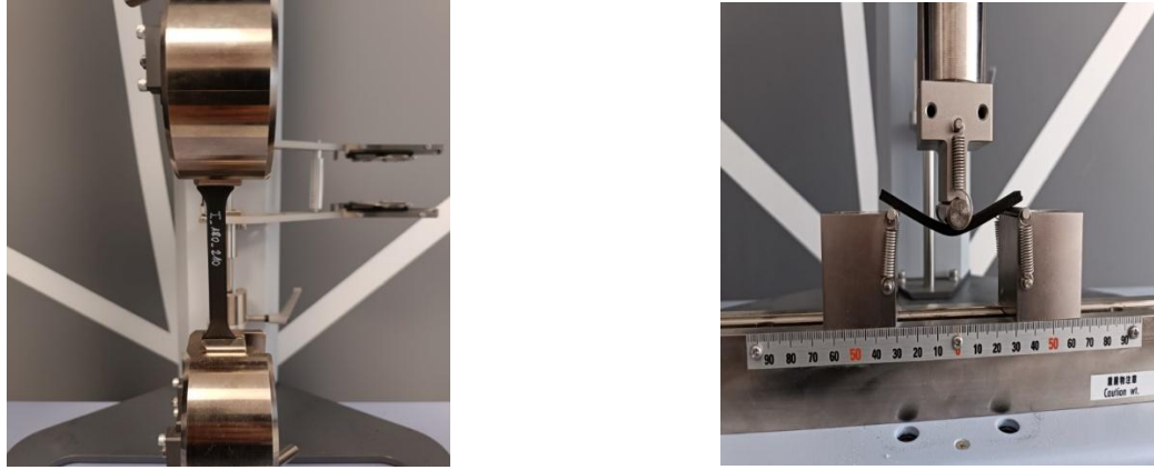
Fig. 6. Tensile (left) and flexural (right) testing setup
