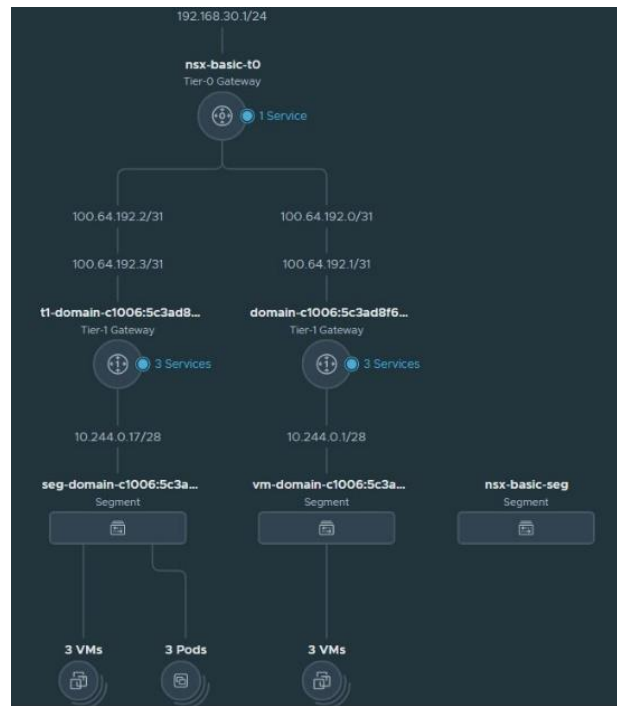
Fig. 2. Network Topology of vSphere with Tanzu Created by NSX-T
