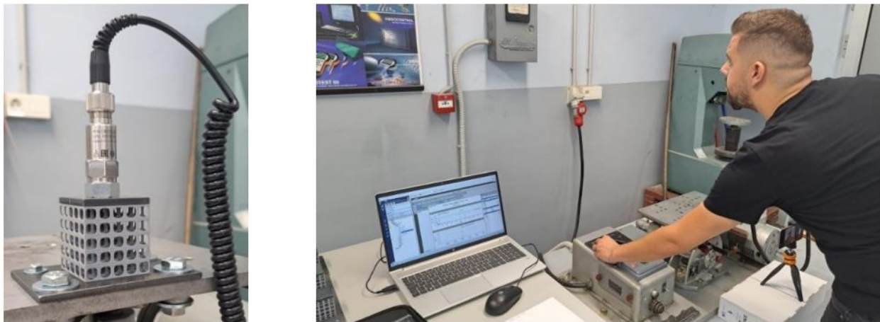
Fig. 7. Vibration sensor positioning (left) and manually adjusted excitation frequency (right)
