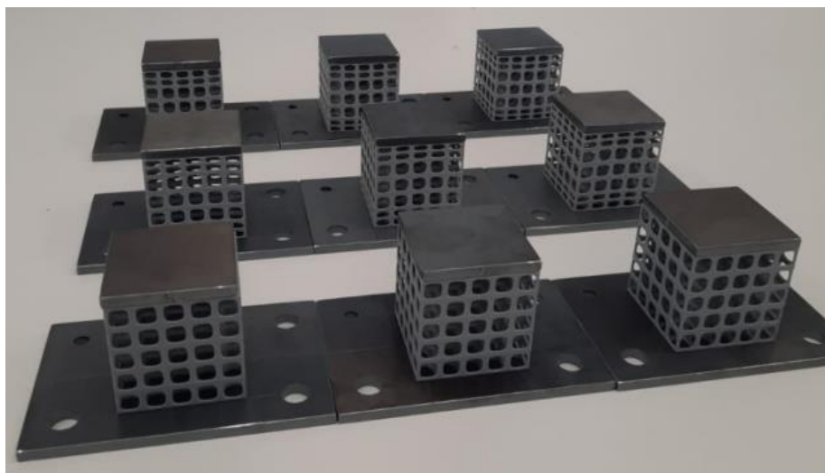
Fig. 5. Samples of series SC – A, SC – B and SC – C glued on steel plates
