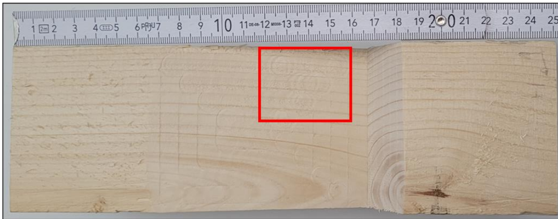
Fig. 3. Occurred chatter marks caused by vibrations and oscillations of the system
