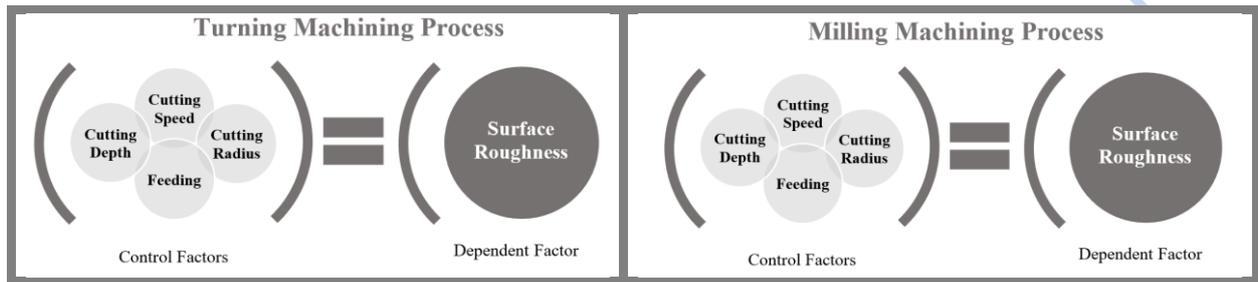
Figure 1. Factors for analysis of relation between surface roughness and cutting parameters
