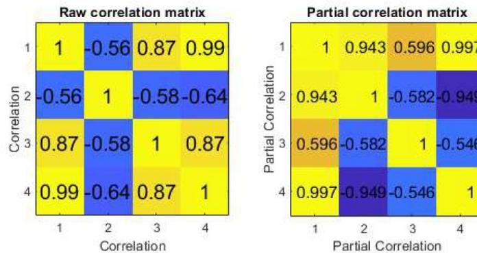
Figure 5. Raw correlation matrix and partial correlation matrix on dependent value as  $R_z$  control factors as cutter speed and feeding for milling machining process
