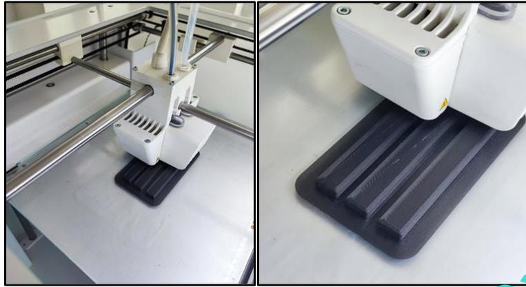
Fig. 3. Printing the specimens
