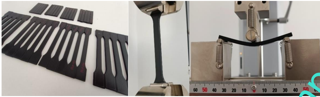
Fig. 5. Tensile and flexural FDM 3D printed specimens
