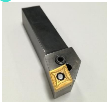
Fig. 1. Toolholder with cemented carbide cutting inserts
