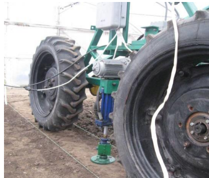
Fig. 1. Technical implementation of turning a gantry tractor
