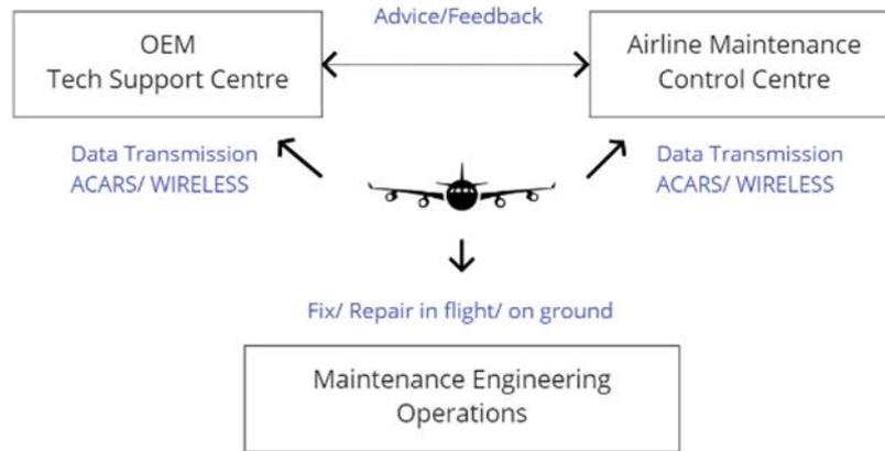
Fig. 2. Aircraft health monitoring schematic.
