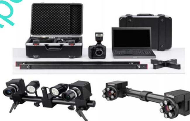
Fig. 3. Passive optical measuring systems (TRITOP, ARAMIS, PONTOS) [1]
