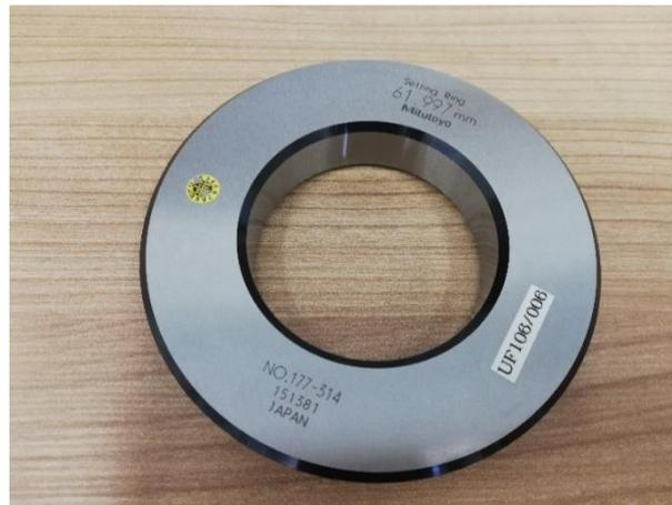
Fig. 2. The calibration ring
