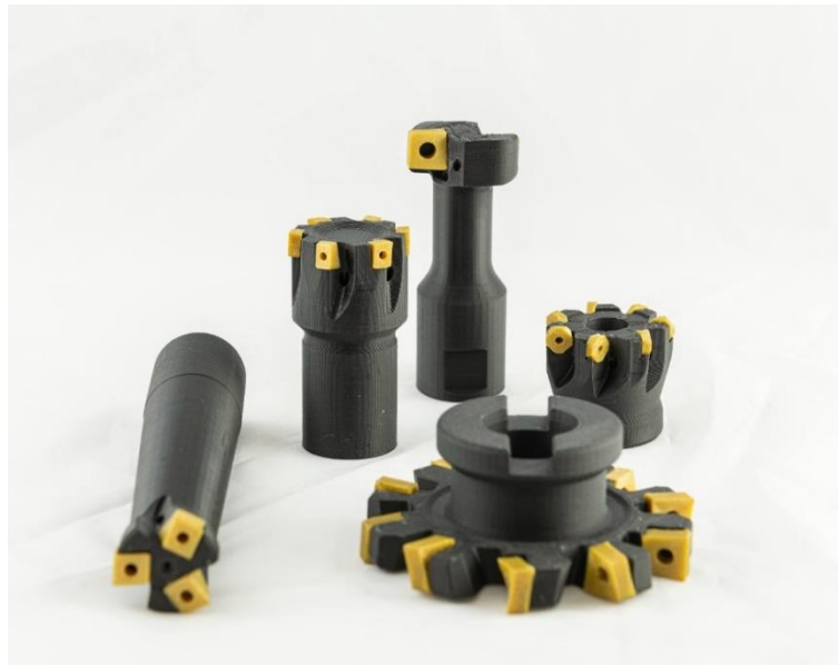
Fig. 5. 3D printed models of milling cutters - different kinds of cutting tools
