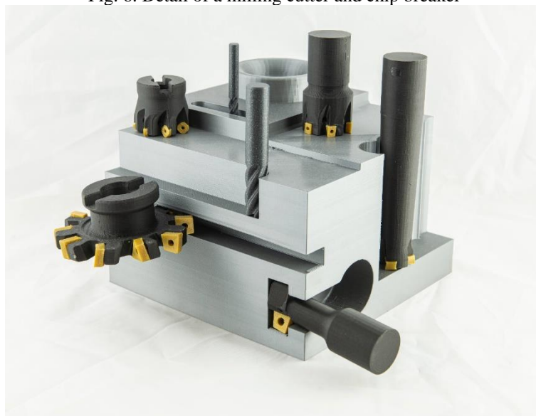
Fig. 7. Application of selected milling cutters on specific surfaces
