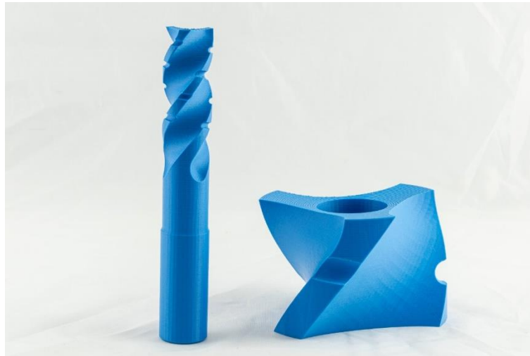
Fig. 6. Detail of a milling cutter and chip breaker
