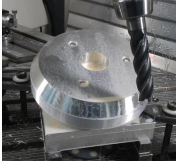
Fig. 6. Machining of the test piece [9]
