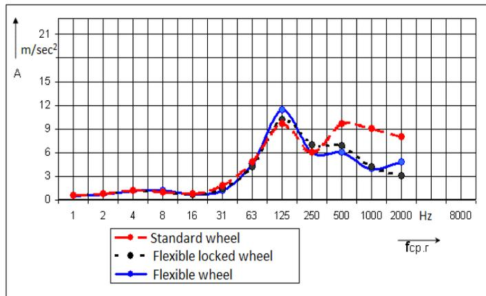
Fig. 10. The spectrum of vibration acceleration amplitudes on the journal box for the three versions of wheel pairs
