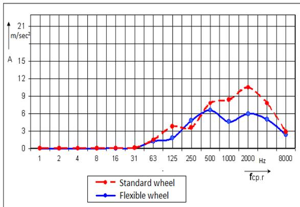
Fig. 8. The frequency spectrum of natural oscillations of the flexible and standard wheels
