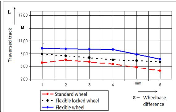
Fig. 6. Dependence of the track passed by bogies on the value of the gauge widening
