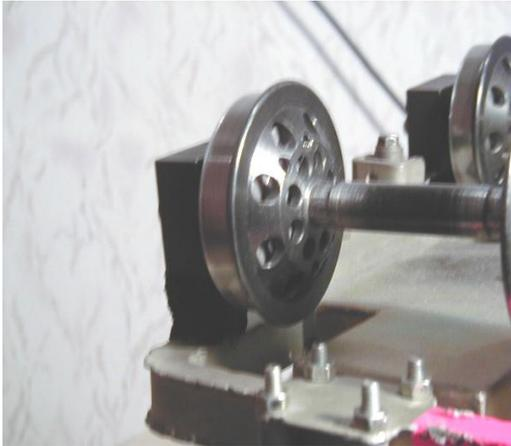
Fig. 2. A wheel pair with independently rotating flexible tires
