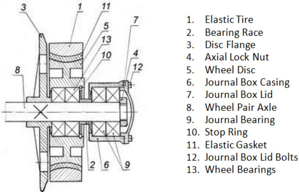
Fig.1. The new wheel pair design
