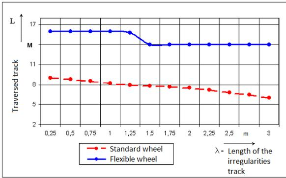
Fig. 5. Dependence of the length of the track traversed by bogies on the number of horizontal irregularities
