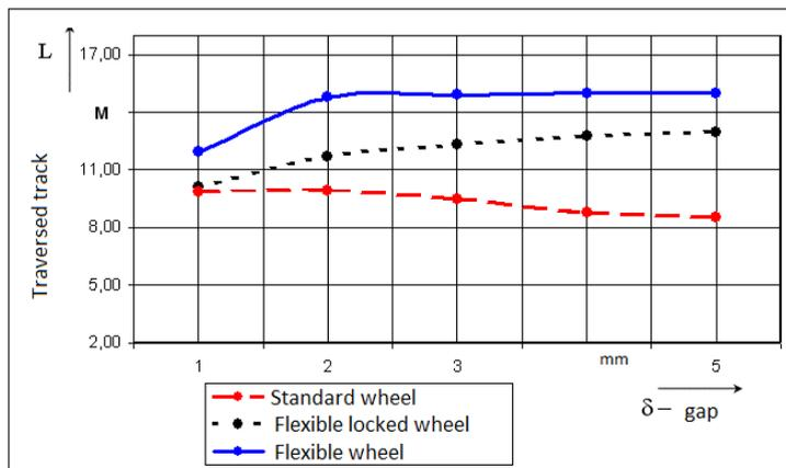
Fig. 7. Dependence of the track traversed by bogies on the value of the wheel pairs misalignment
