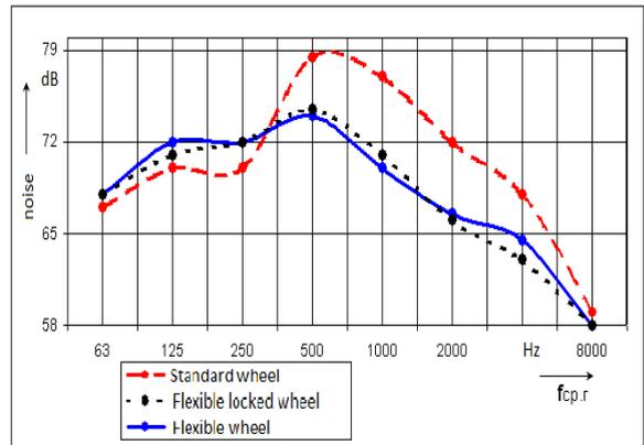
Fig. 9. The frequency spectrum of the sound pressure amplitudes for the three versions of wheels
