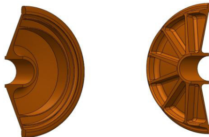
Fig. 7. (a) The flange disc with annular ribs (rear view); (b) The flange disc with radical ribs (rear view).
