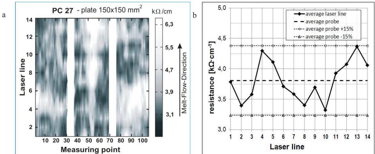
Fig. 6. Resistance values; (a) over the surface of the plate in the laser lines; (b) average values in the laser lines.
