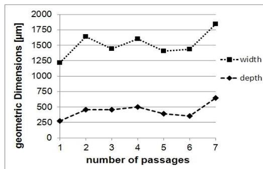
Fig. 8. Changes to the line width and depth through multiple passages.
