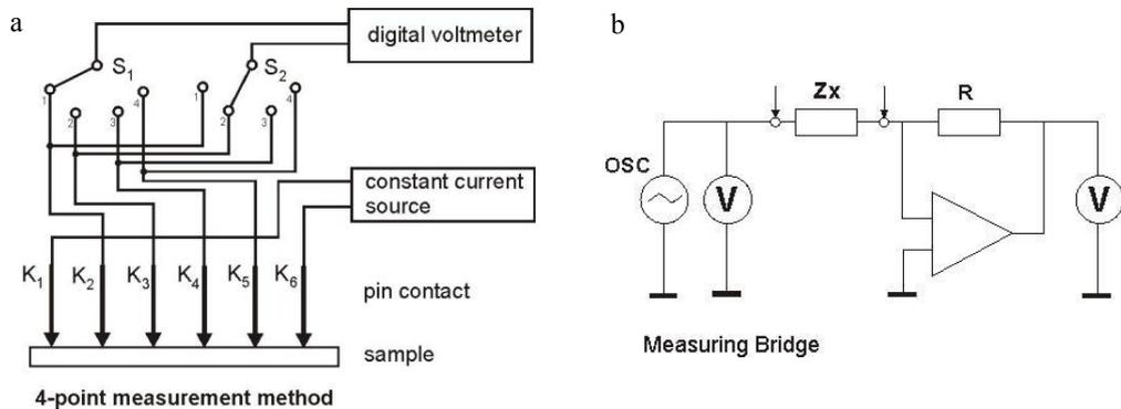
Fig. 2. Resistance Measurement Setup; (a) 4-point measuring method; (b) measuring bridge.
