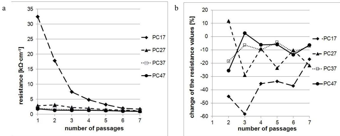
Fig. 7. Change of the values through multiple passages; (a) resistance absolut; (b) in percent.
