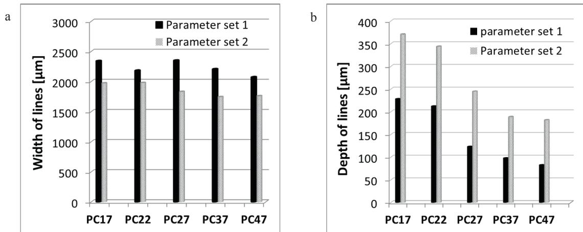
Fig. 4. Geometry of laser activated lines; (a) Width of lines; (b) Depth of lines.
