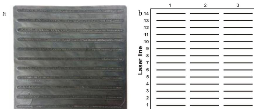
Fig. 1. Arrangement of laser lines; (a) Photograph of (60x60x2.6) mm<sup>3</sup> Standard – plate ; (b) Schematic representation of (150x150x2.6) mm<sup>3</sup> plates.
