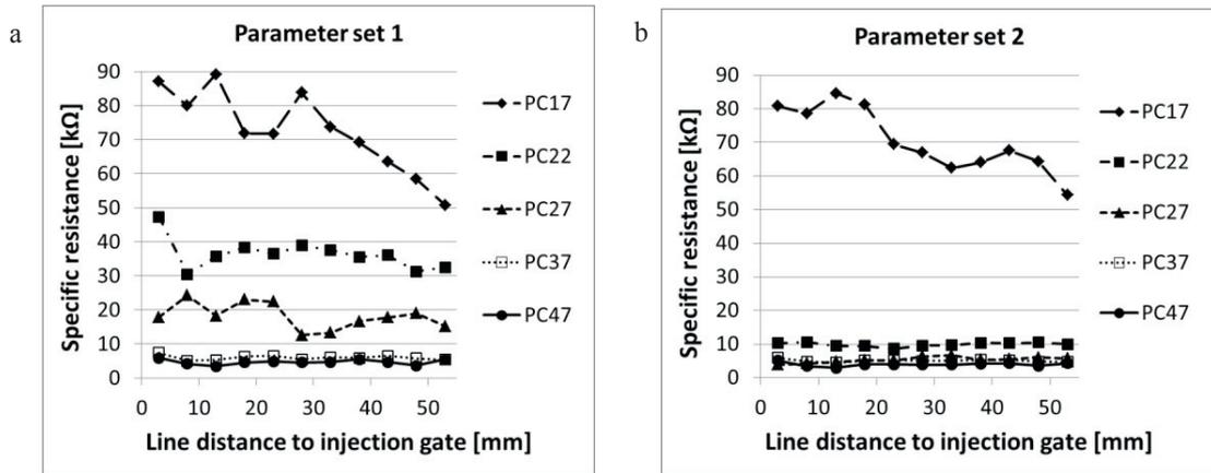
Fig. 5. Resistance of laser activated lines; (a) Parameter set 1; (b) Parameter set 2.
