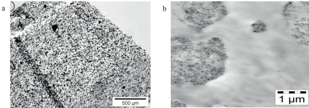
Fig. 3. Optical and transmission electron microscopy representing the blend morphology of sample PC22 [10]; (a) Optical micrographs of thin-section; (b) TEM-Image.
