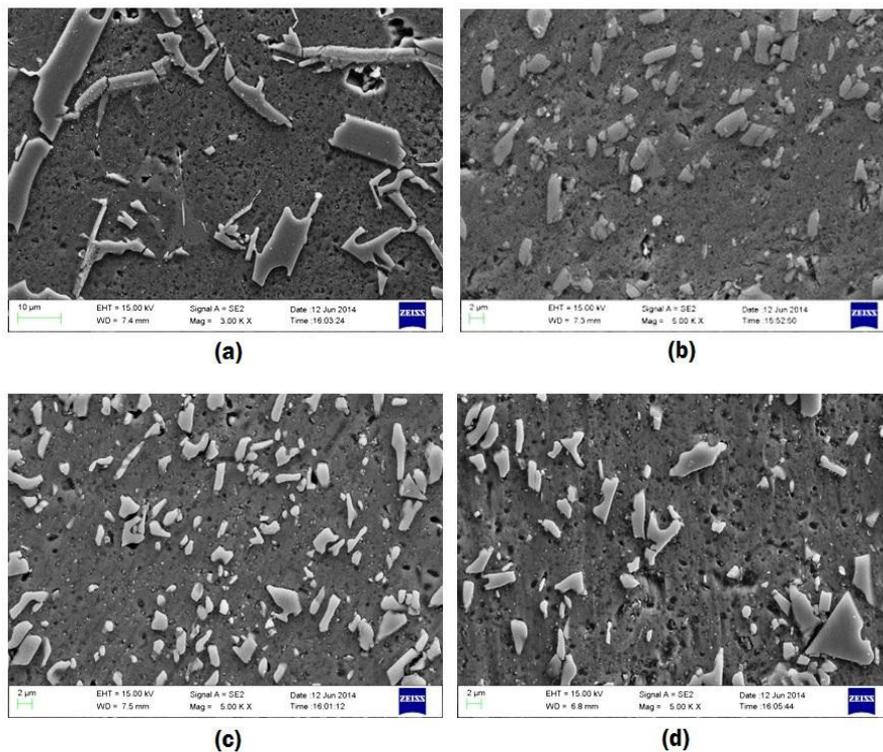
Fig. 6. SEM images (a) Base material; (b) FSPed at 26 mm/min; (c) FSPed at 40 mm/min; (d) FSPed at 60 mm/min.
