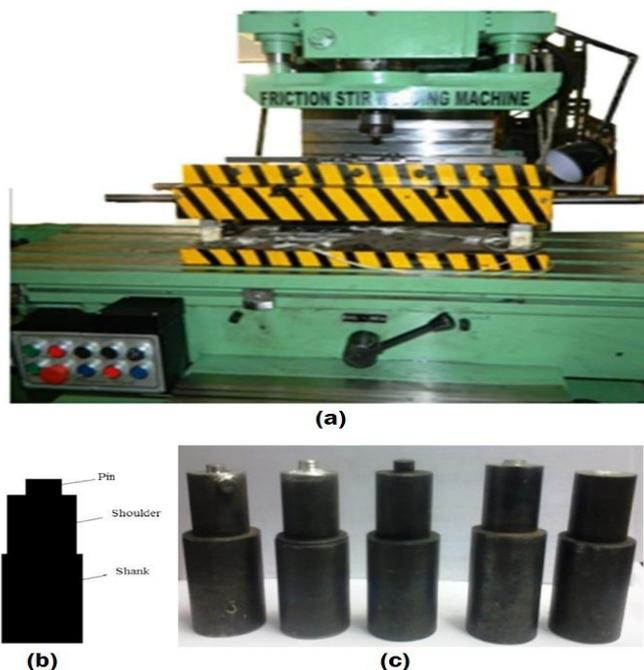
Fig. 3. (a) Photograph of Friction stir welding machine; (b) Designed tool geometry; (c) Various tool made for friction stir processing for Al-17%Si cast alloy .
