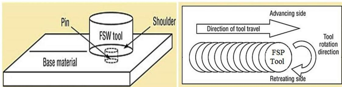
Fig. 2. A schematic diagram of friction stir processing.
