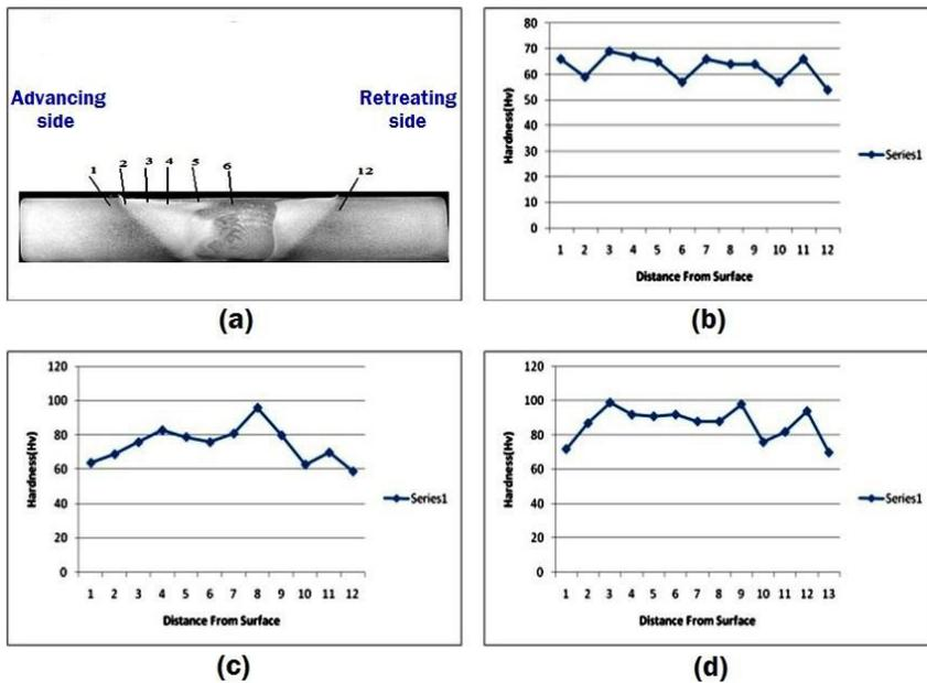
Fig. 10. (a) locations of hardness analysis; (b), (c) and (d) Microhardness of FSPed cast Al-17wt% Si alloy developed using 664 rpm tool rotation speed and 26, 40, and 60 mm/min welding speed.
