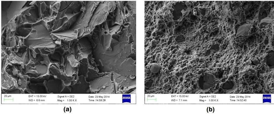
Fig. 9. Fracture surfaces of FSPed samples (a) base material and (b) FSPed sample at 26 mm/min and 664 rpm.
