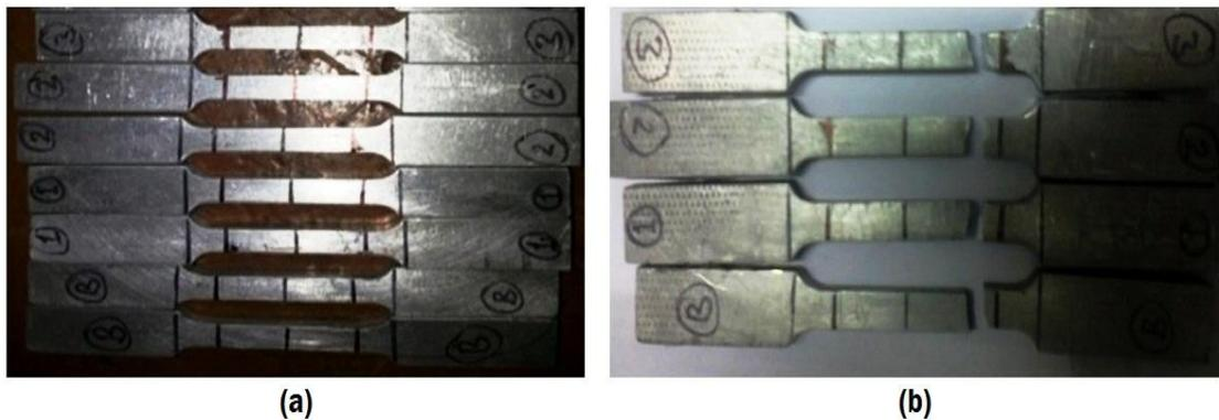
Fig. 8. Tensile samples of FSPed cast Al-17wt% Si alloy at 664 rpm tool rotation speed and 26, 40, 60 mm/min tool transverse speed.
