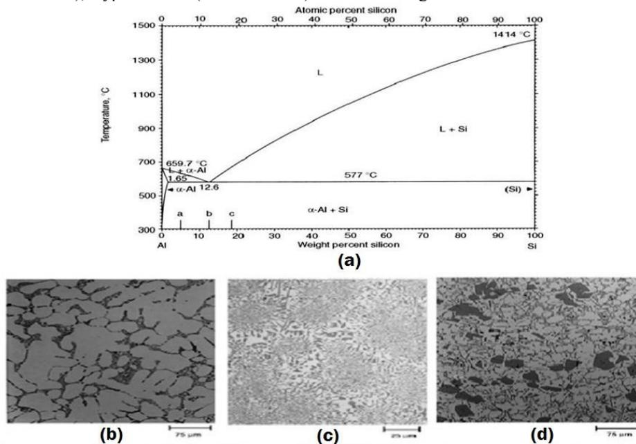
Fig. 1. (a) Al-Si equilibrium diagram of Al-Si alloy; (b) Microstructure of hypoeutectic alloy (1.65-12.6 wt% Si); (c) Microstructure of eutectic alloys (12.6% Si); (d) Microstructure of hypereutectic alloy (>12.6% Si) [7].
