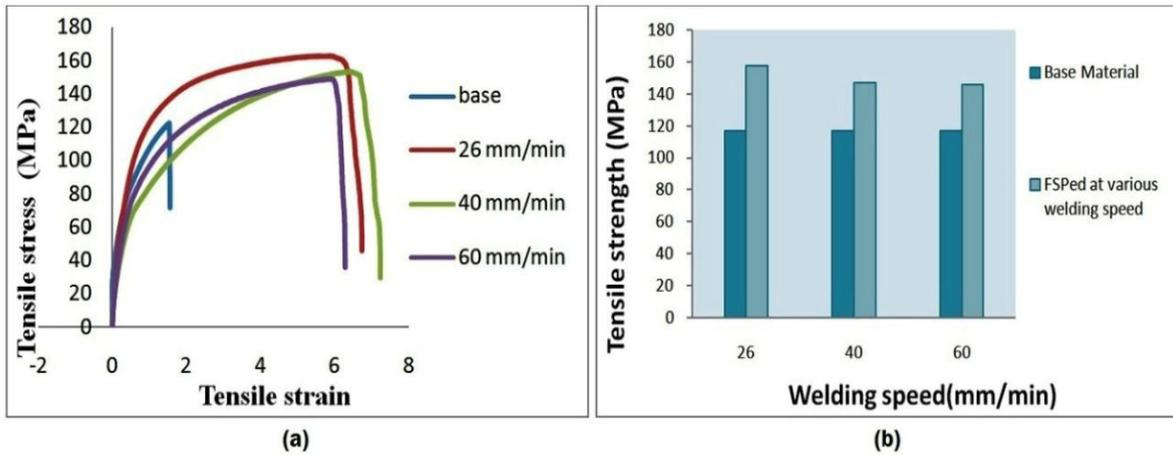
Fig. 7. (a) Stress verses strain in base and FSPed samples at various process parameters;
