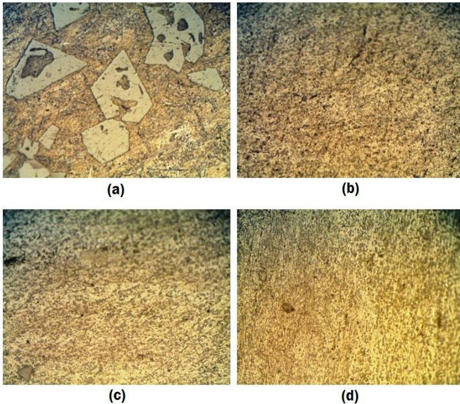
Fig. 5. Friction stir processed zone and cross sectional view of micrographs at (a) 664 rpm and 26 mm/ min; (b) 664 rpm and 40 mm/min; (c) 664 rpm and 60 mm/min.
