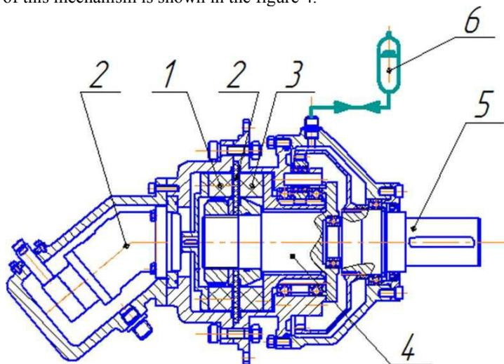
Fig. 4. Rotation sealed lead-in unit and planetary gearbox combined as a single mechanism.
