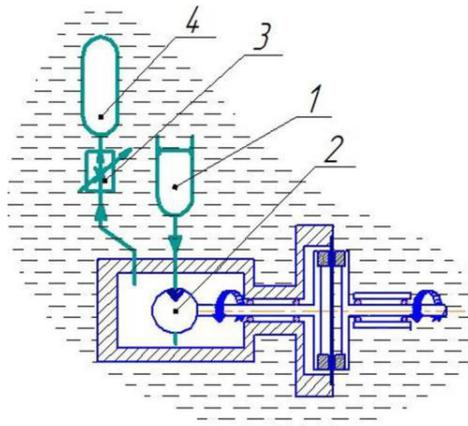
Fig. 1. Rotary drive using hydrostatic pressure
