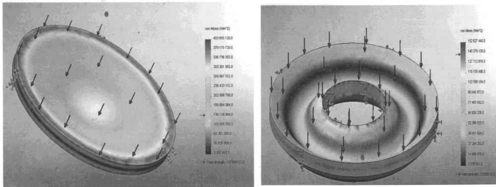
a) Fig. 3. Results of stress and deformation calculations of (a) tough membrane and (b) circular membrane.
