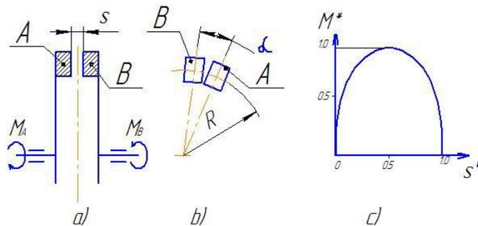
Fig. 2. Dependence of relative torque from angle of deviation of the magnets.
