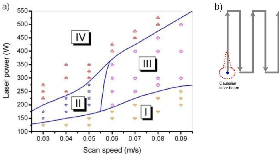
Fig. 2. a) Dependency of the structure on the procedural parameters; b) Procedure of the powder laser scanning. [2]
