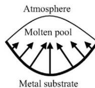
Fig. 8. Diagram of the solidification of melted pool during SLM process. [8]
