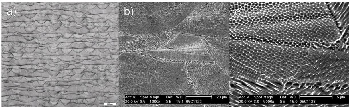
Fig. 1. EOS CobaltChrome- MP1; a) 10x enlarged; b) 1000x SEM; c) 5000x SEM. [1].
