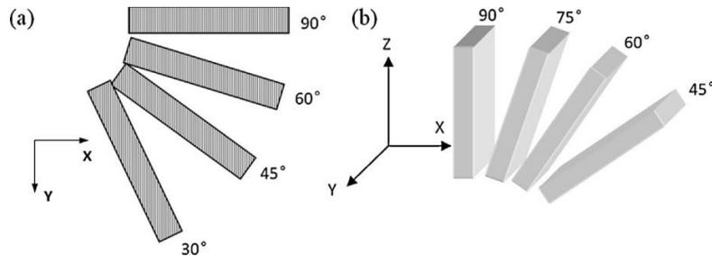
Fig. 6. Manufacturing strategy of the tensile samples: a) horizontal; b) vertical. [8]
