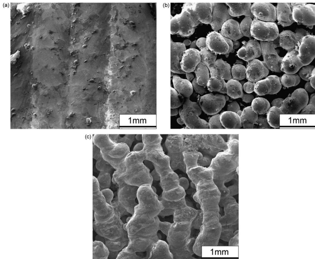
Fig. 3. The structure of molten samples; a) full consistent surface; b) surface with balling phenomenon; c) porous structure. [2]
