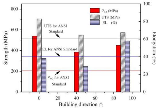
Fig. 7. Tensile properties of SLM specimens at varying building directions. [5]
