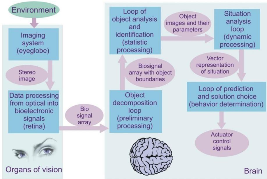
Fig. 1. Functional schematic of binocular vision data processing.
