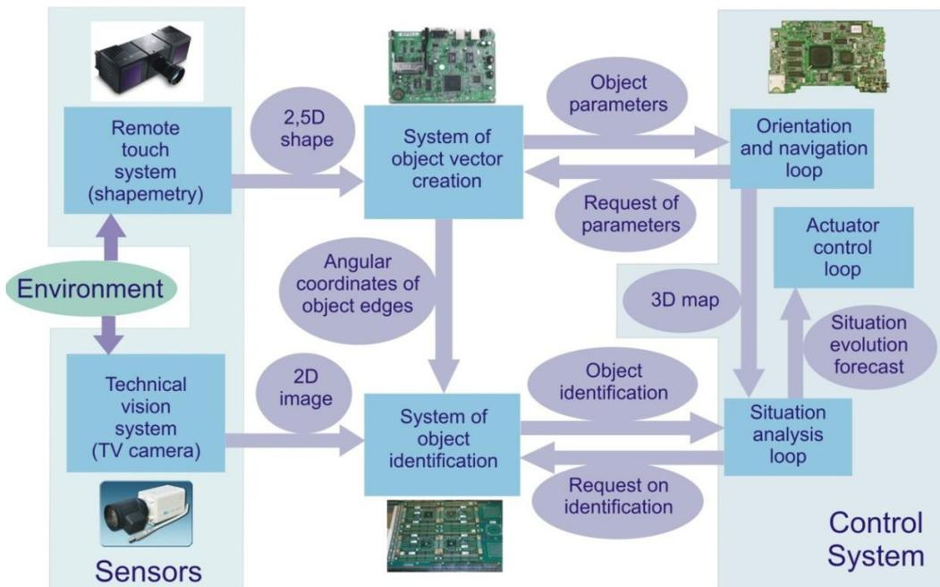
Fig. 2. Architecture of visual data processing for autonomous robotic system.
