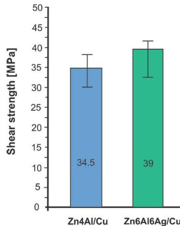
Fig. 5. Shear strength of soldered joints with solders Zn4Al a Zn6Al6Ag.
