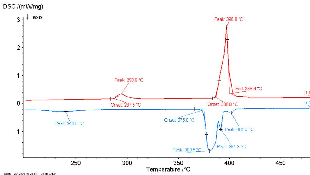
Fig. 2. DSC analysis of Zn6Al6Ag solder.
