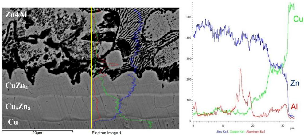
Fig. 3. Line EDX analysis of  $\text{Cu/Zn4Al}$  soldered joint and concentration profiles of  $\text{Cu}$ ,  $\text{Zn}$ ,  $\text{Al}$  elements on  $\text{Cu/Zn4Al}$  boundary.
