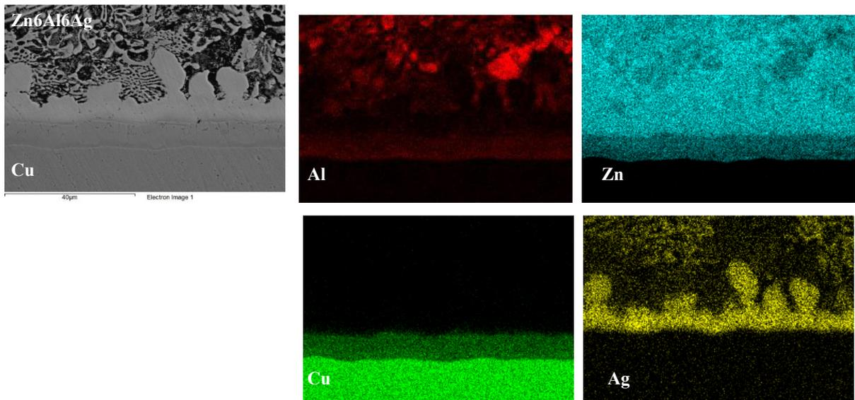
Fig. 4. Planar distribution of elements on the  $\text{Cu/Zn6Al6Ag}$  boundary.
