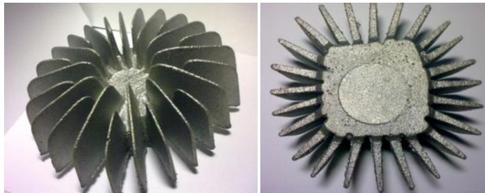
Fig. 10. Sample Chart Fan heads after casting.
