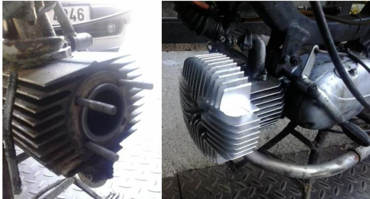
Fig. 7. Mounting the head for motorcycle Jawa 50.
