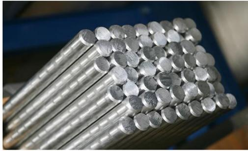
Fig. 8. The Aluminium rods EN AW 7075 [5].
