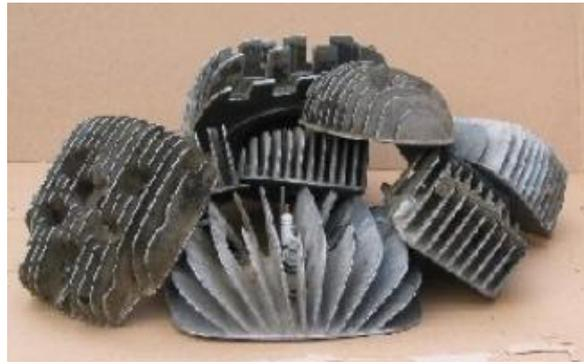
Fig. 3. Various structural solutions of the cooling heads for motorcycles Jawa [3].
