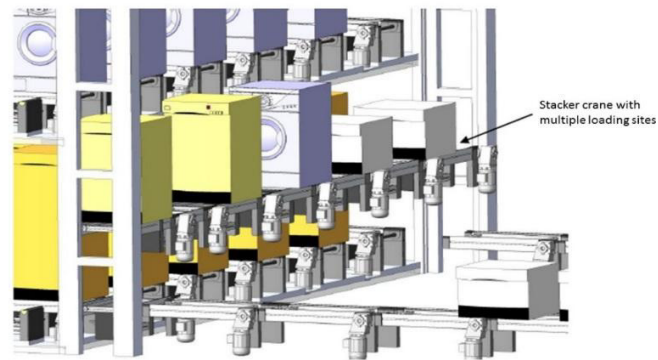
Fig. 7. Outlet of products using stacker crane.
