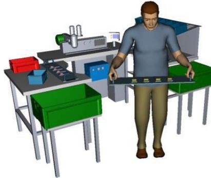
Fig. 3. Position during transferring –Tecnomatix Jack visualization.
