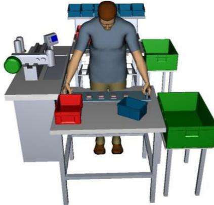
Fig. 4. Initial posture for clamping jig lifting – Tecnomatix Jack visualization.
