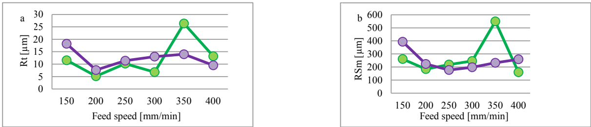
Fig. 6 (a) Influence of feed speed on roughness Rt; (b) Influence of feed speed on surface roughness RSm.
