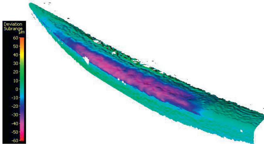
Fig. 9. Differential analysis of the cutting edge.
