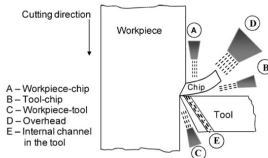
Fig. 1. Basic direction of coolant applications taken from [2].
