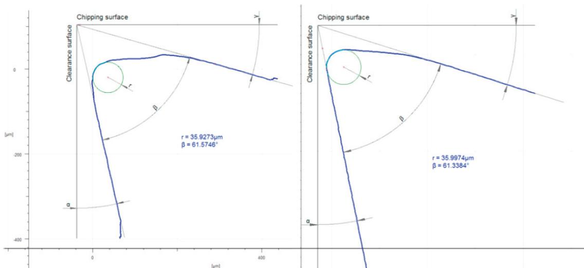
Fig. 10. 2D measurement - worn and unworn cutting edge.
