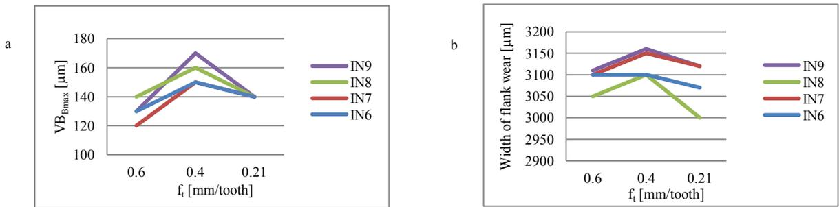
Fig. 7. (a) Influence of  $v_c$  on  $VB_{Bmax}$ ; (b) Influence of  $f_t$  on width of flank wear.
