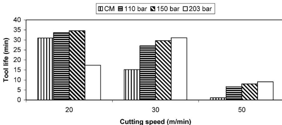
Fig. 2. Tool life - machining of INCONEL 718 at various coolant pressures at feed rate of 0.3 mm/rev - taken from [1].
