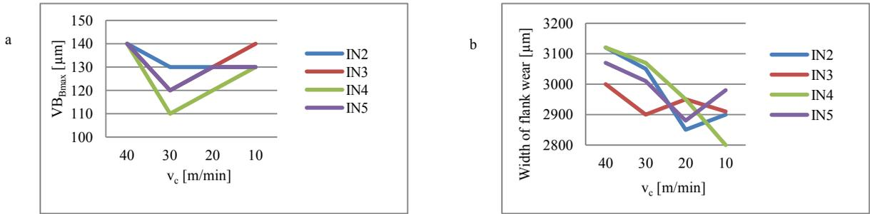
Fig. 6. (a) Influence of  $v_c$  on  $VB_{Bmax}$ ; (b) Influence of  $v_c$  on width of flank wear.
