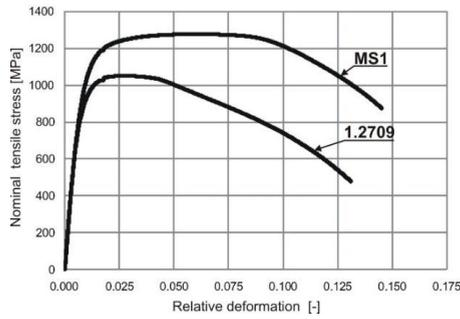
Fig. 3. Nominal Tensile Stresses of Tested Materials (1.2709, MS1).
