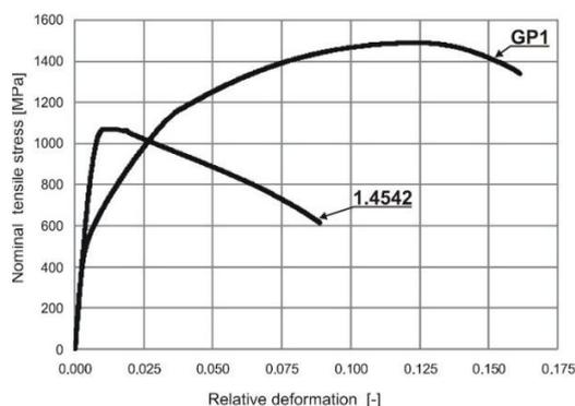
Fig. 2. Nominal Tensile Stresses of Tested Materials (1.4542, GP1).
