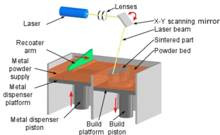
Fig. 1. Principle of DMLS Method [3, 14].
