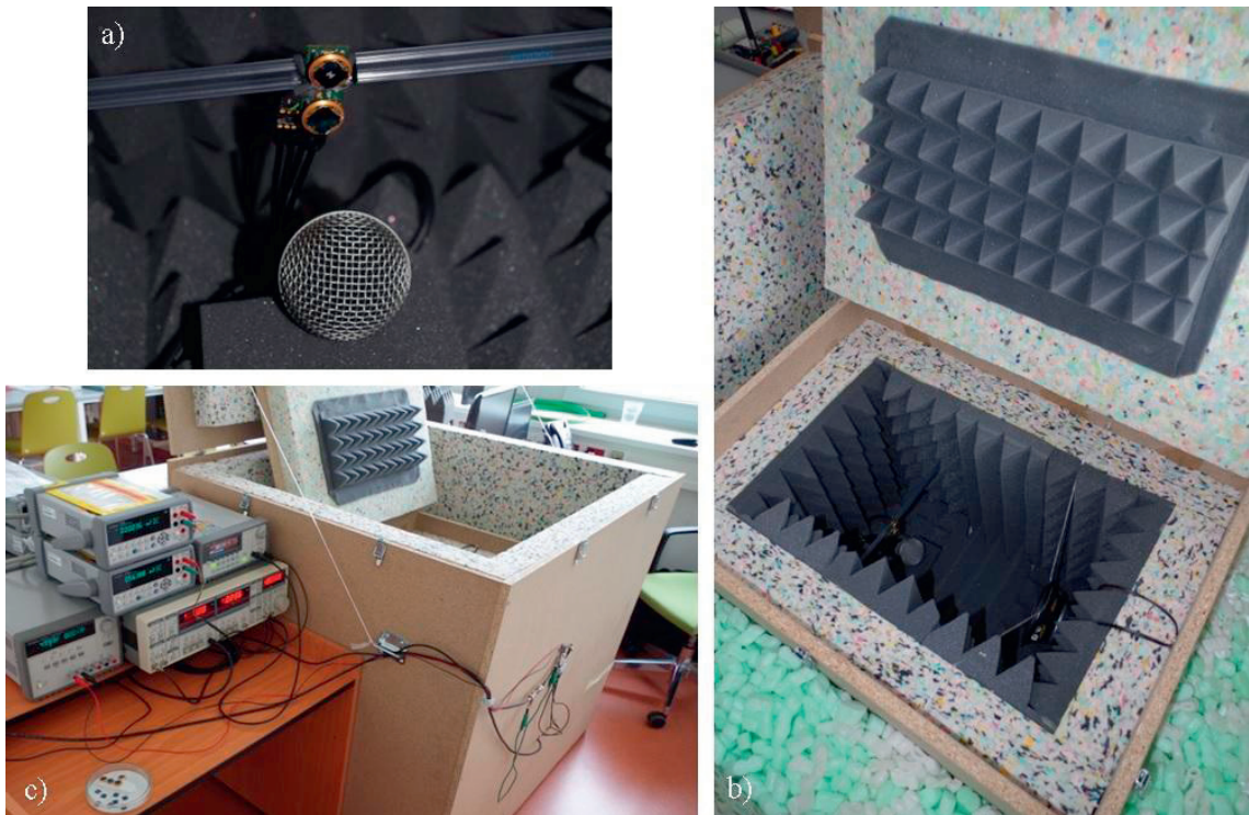
Fig. 5. a) MEMS sensor and reference microphone, b) the anechoic box and c) the measurement setup detail.
