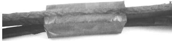
Fig. 6. Breaking of vulcanization joined test pieces in the case of using ultrasonic energy.
