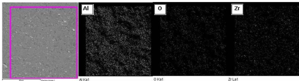
Fig. 2. SEM images of fracture surface (back-scattered electrons mode) of  $Al_2O_3$ -t- $ZrO_2$  composite ceramics with 5 wt. % of t- $ZrO_2$ ; X-ray mapping micrographs of different elements: Al, O and Zr.
