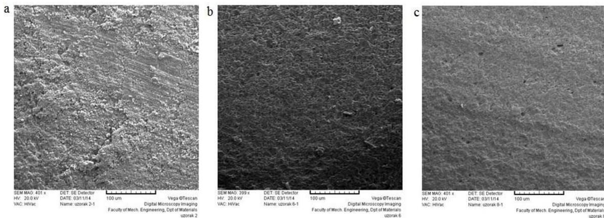
Fig. 6. SEM images of prepared samples before erosion: (a) monolithic Al<sub>2</sub>O<sub>3</sub>; (b) composite Al<sub>2</sub>O<sub>3</sub>-t-ZrO<sub>2</sub> containing 5 wt.% of t-ZrO<sub>2</sub>; (c) composite Al<sub>2</sub>O<sub>3</sub>-t-ZrO<sub>2</sub> containing 10 wt.% of t-ZrO<sub>2</sub>.
