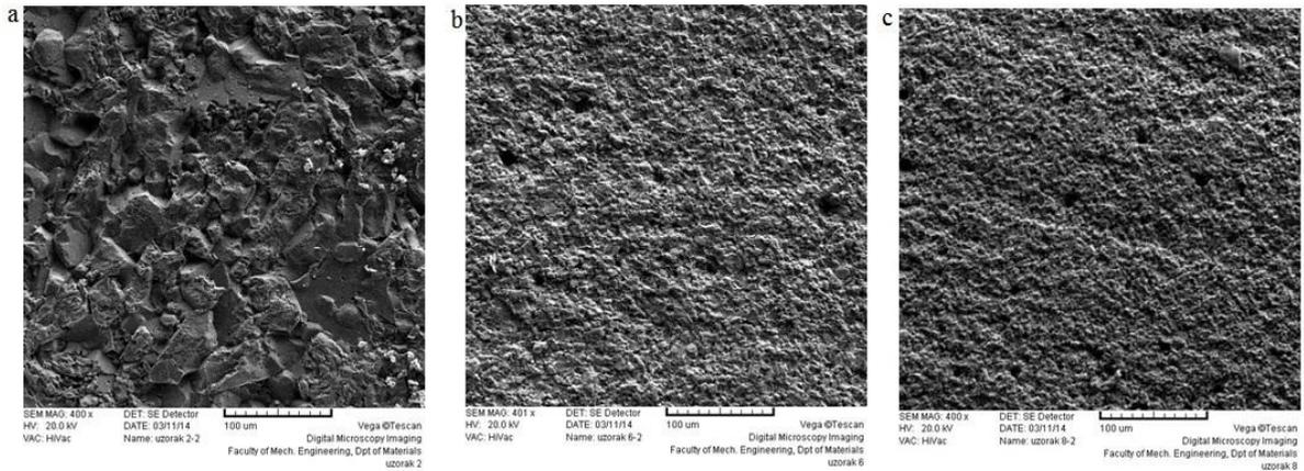
Fig. 7. SEM images of prepared samples after erosion at 30°: (a) monolithic Al<sub>2</sub>O<sub>3</sub>; (b) composite Al<sub>2</sub>O<sub>3</sub>-t-ZrO<sub>2</sub> containing 5 wt.% of t-ZrO<sub>2</sub>; (c) composite Al<sub>2</sub>O<sub>3</sub>-t-ZrO<sub>2</sub> containing 10 wt.% of t-ZrO<sub>2</sub>.
