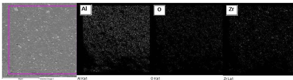
Fig. 3. SEM images of fracture surface (back-scattered electrons mode) of  $Al_2O_3$ -t- $ZrO_2$  composite ceramics with 10 wt. % of t- $ZrO_2$ ; X-ray mapping micrographs of different elements: Al, O and Zr.
