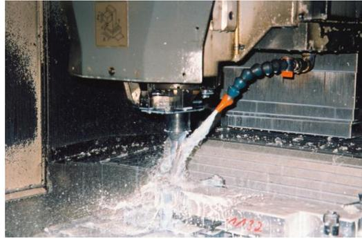
Fig. 1. Flood cooling.
