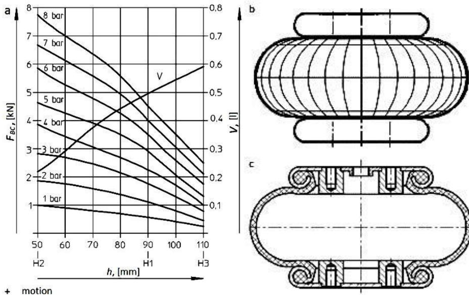
Fig. 1. (a) load bearing characteristics, bulk property; (b) design; (c) construction of bellow actuator.
