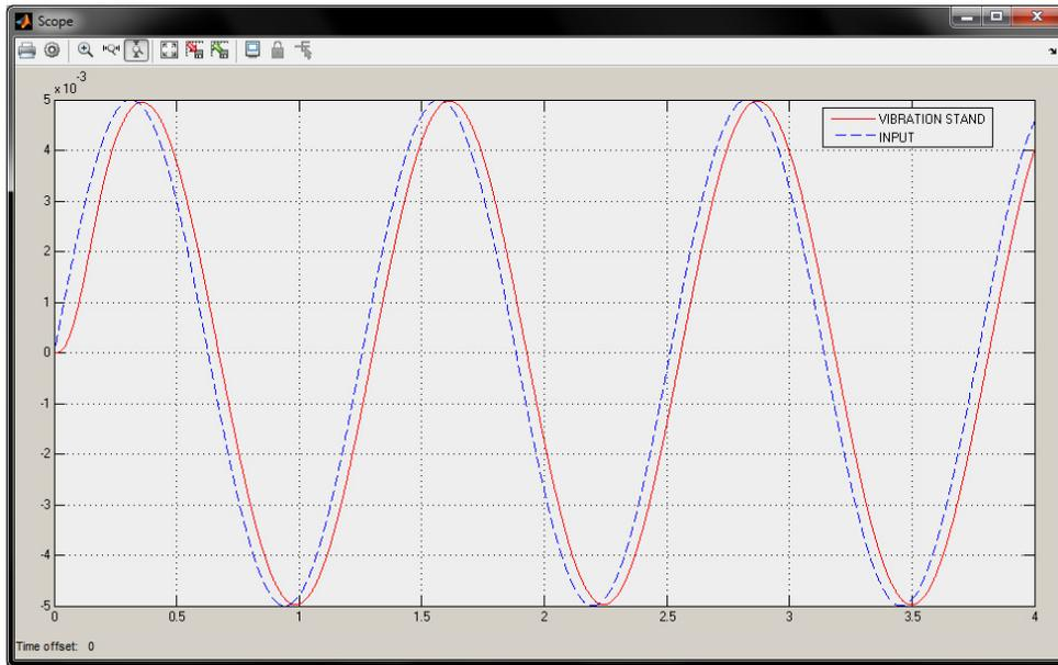
Fig. 3. Sin wave reaction of a vibration stand actuator.
