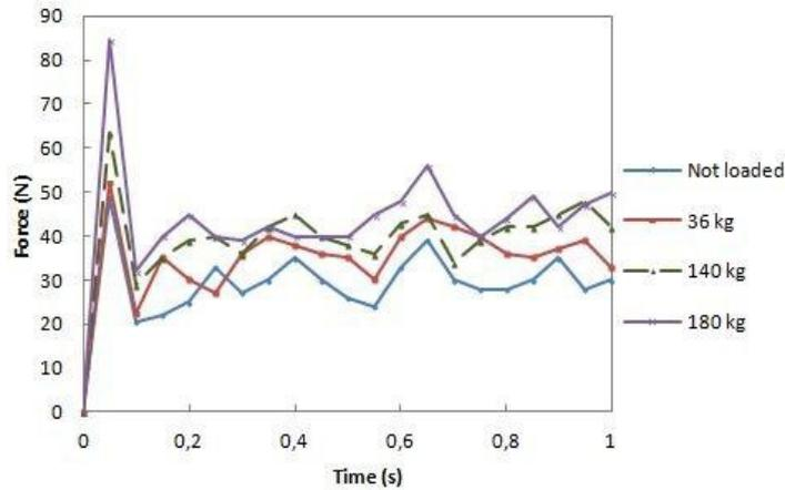
Fig. 10. Friction behaviour of the slide on four carriages with no preloads.
