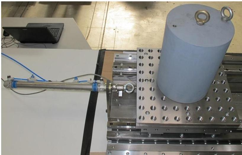
Fig. 9. Friction experimental set-up of the slide under a load of 140 kg.
