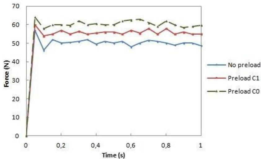
Fig. 7. A comparison between friction behaviour curves of the three preload classes under a load of 160 kg.
