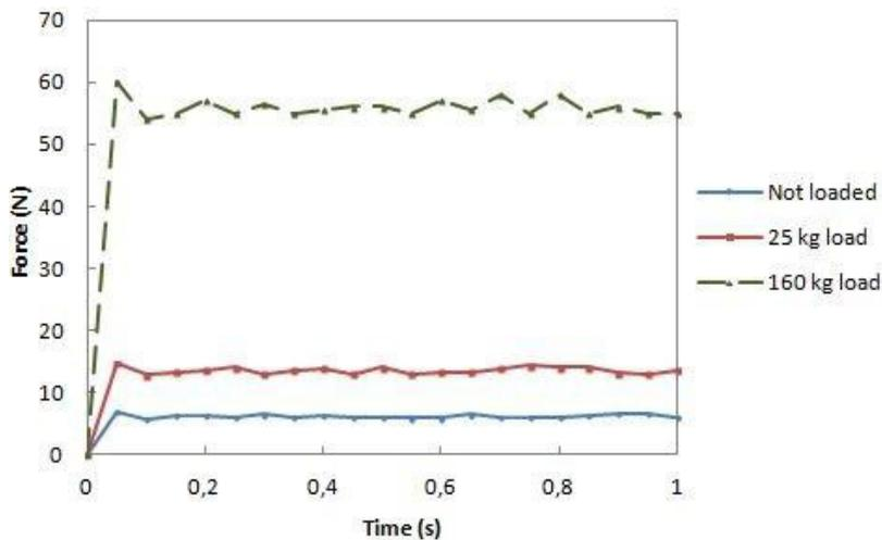
Fig. 5. The force-time curve of the tests for the carriage with light preload (C1).
