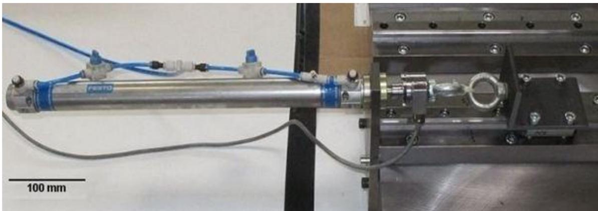
Fig. 1. The experimental set-up of the stick-slip effect and friction tests.
