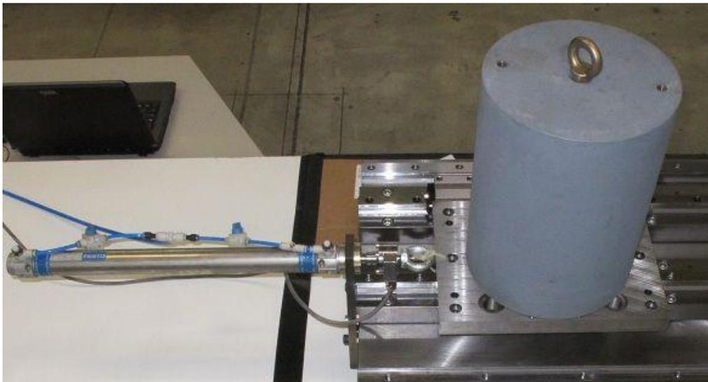
Fig. 3. The experimental set-up under the external load of 160 kg.
