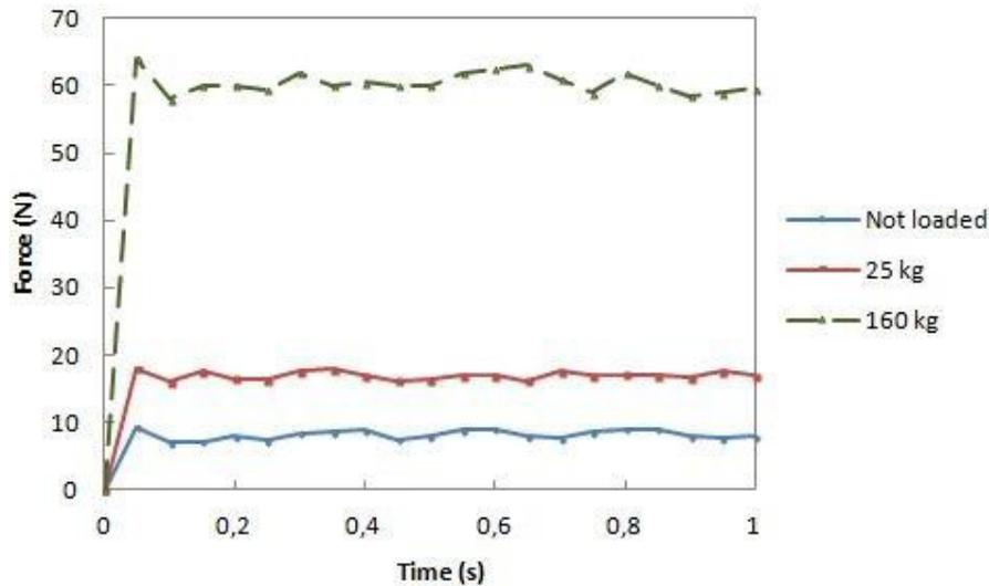
Fig. 6. The force-time curve of the tests for the carriage with medium preload.
