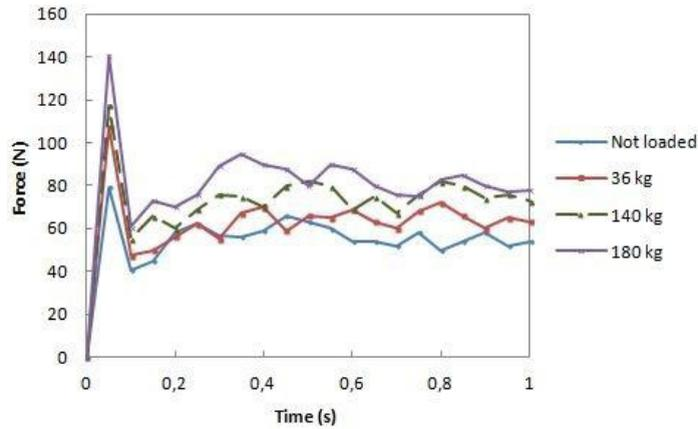
Fig. 12. Friction curves of the slide on carriages with medium preload.
