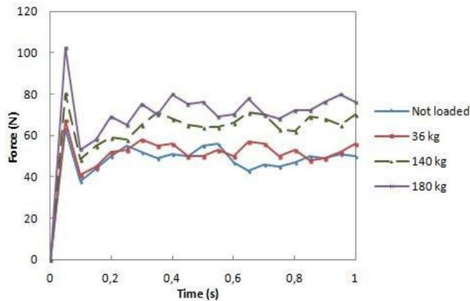
Fig. 11. Friction behaviour of the slide on four carriages with light preload.
