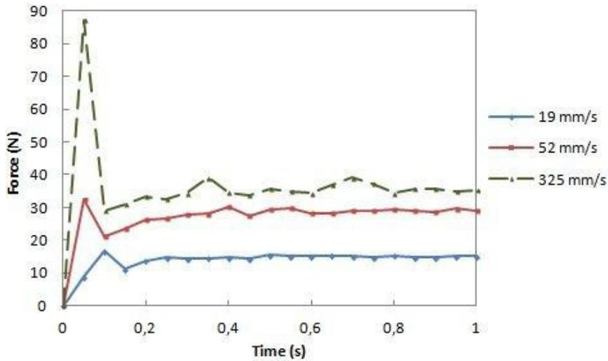
Fig. 8. The friction curve of the guide with light preload and different velocities.
