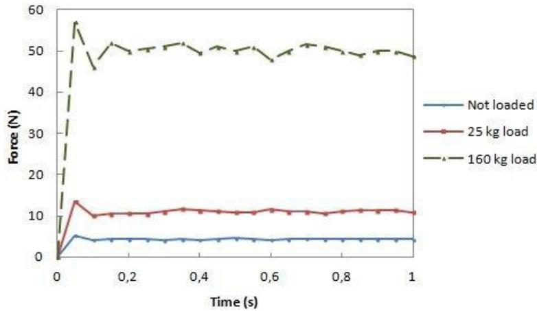
Fig. 4. The force-time curve of the friction tests for the carriage without preload.
