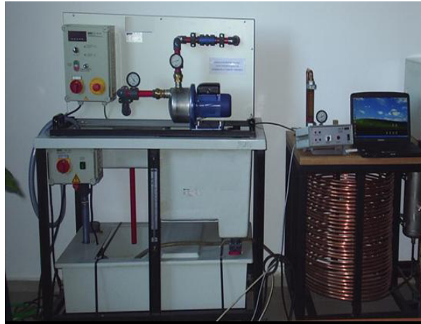
Fig. 2. Experimental stand for pump performance study (FIFIM-USAMVB Laboratory).
