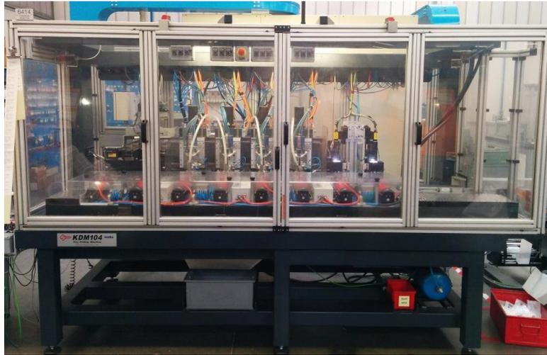
Fig. 1. CNC milling machine for key cutting.
