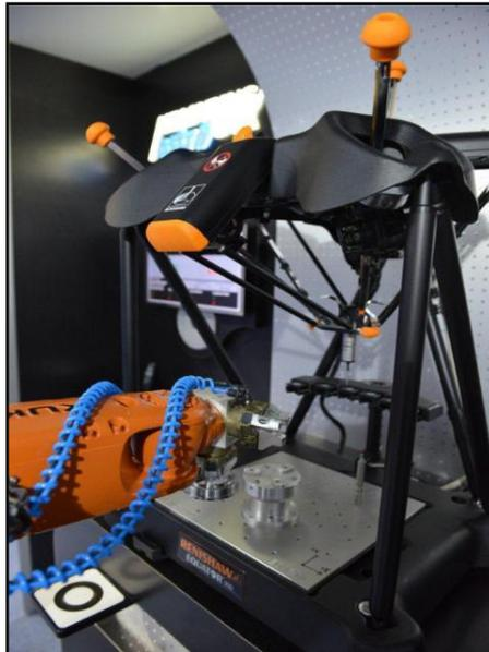
Fig. 1. Measuring device Equator [5].
